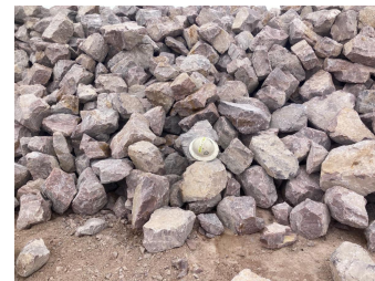
Finished Rip Rap product in stockpile using a hard hat as size reference
