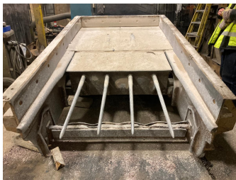
Rip Rap screener from the Dells East Primary Plant
